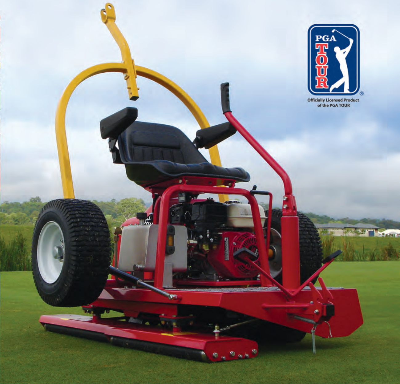
Spikers – 11x8 points to a depth of 30mm (1.25")
