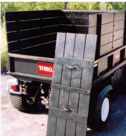
This view shows the tailgate assembly and the "tension" chain that keeps the back and sides from rattling during transport. Photo by Darren Davis.
