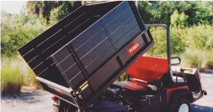
Creating a high-sided wagon accessory for the Toro Workman cost less than $100. Photo by Darren Davis.
