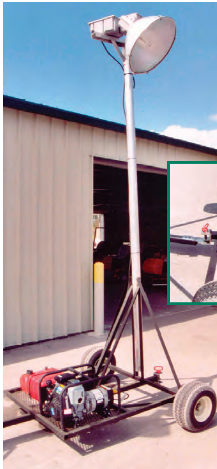
The grow lights are attached to an aluminum pole that can be raised up to 12 feet.
