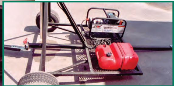
The lights are powered by a 2700-watt generator with fuel supplied by a 6-gallon marine fuel tank, both mounted on the bed of the trailer.
