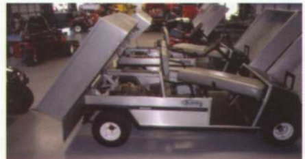
Photo 4. Opening up beds and cowlings helps equipment to dry quickly and completely to help prevent corrosion.
