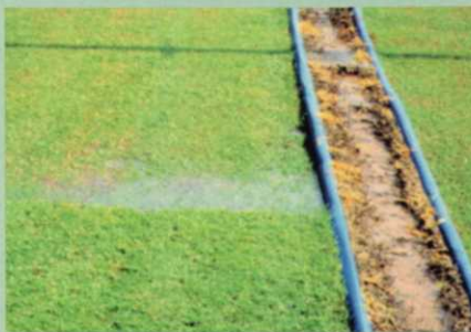
Runoff from rainfall simulators on sloped fairway height plots is stopped by 3" high rough buffer zone. Note standing water that will now infiltrate slowly. Oklahoma State research plots. Photo by Jim Baird.
