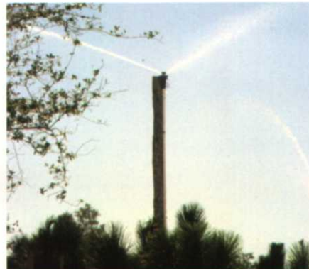
Toro 670 heads were mounted on trimmed pine tree trunks to cover nursery holding area. Elevated position insured all plant material received adequate watering. Photo by Darren Davis.
