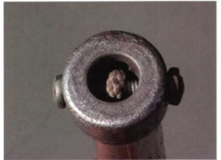
A small bolt acts as a stopper for the cord lasso on the end of the snake stick. Photo by Bill Davidson, Jr.
