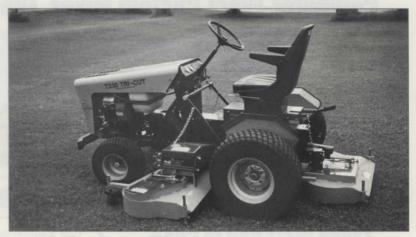
The Tri-Cut Mower has three floating 17" x 31" decks designed to follow turf contours. It performs well even on the hills and valleys, and is great in the wide-open spaces. It is powered by a 23 HP Briggs and Stratton engine and produces an overall cutting width of 80"
