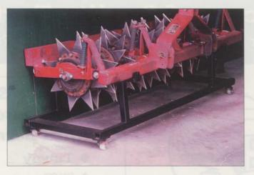
The finished dolly on casters. Stored out of the way when not in use, but easy to move around for blade changes or hook ups to tractors. Photo by Darren Davis.
