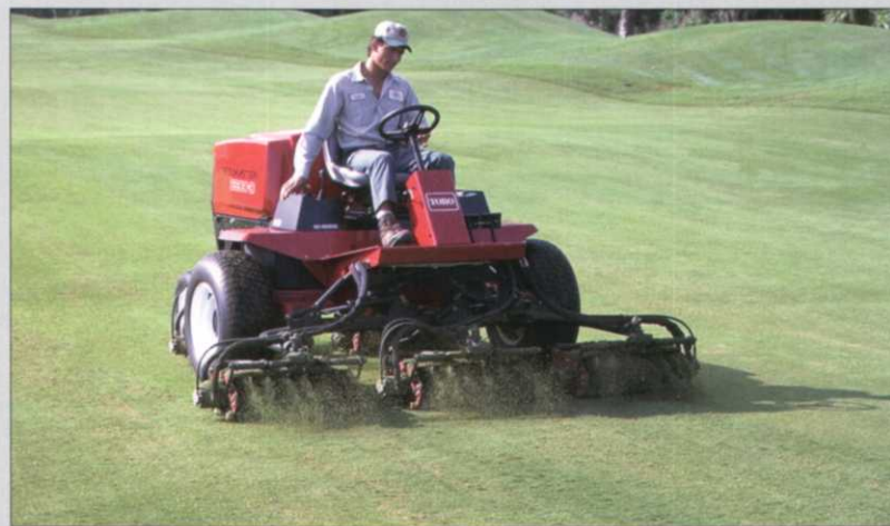
Making one-way passes down a fairway against the grain, a tractor-mounted, street-sweeper broom, above, stands the turf up and then double-cutting the fairways, below, mows off the grain, producing good lies on upright grass
