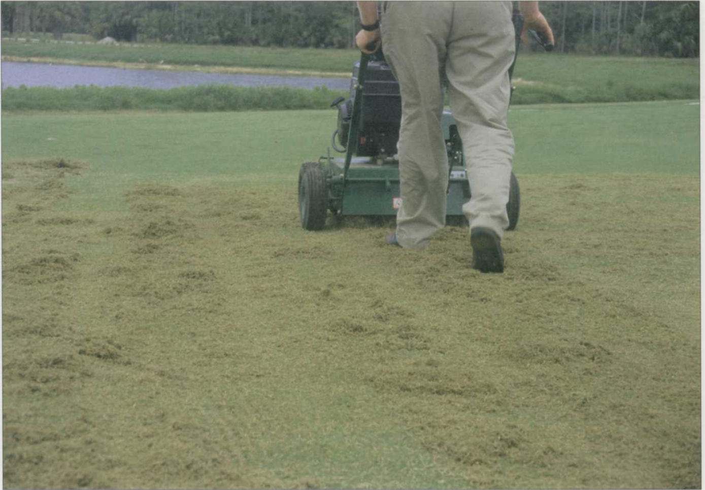
Once a year, usually in May, an aggressive Mat-A-Way verticutting is performed to control potential thatching. Photo by Matt Taylor.
