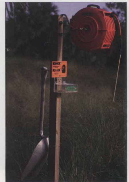
A slightly more advanced blow-off station utilizing a retractable hose reel, a warning sign, and a safety glasses holder. The shovel mounted behind the support pole is used to clean up any build up of clippings in the area. Photo by Darren Davis.
