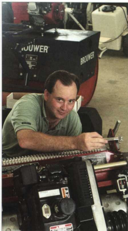
You never know what a UF IFAS Extension professor will be doing when you drop in. Dr. Bryan Unruh adjusts the bedknife on a Toro walk mower at the Milton Campus, also known as the West Florida Research and Education Center. Photo by Joel Jackson
