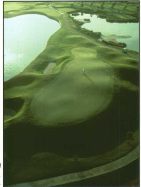
From behind Grand Harbor #7. Lined and walled effluent receiving lake to the right. Percolation pond in use of the left.
