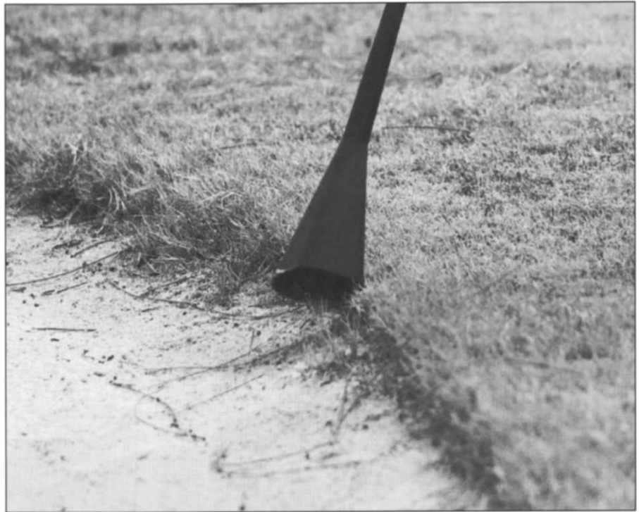
An inverted square-mouthed funnel attached to a spray wand gives a nice crisp edge when chemically treating bunkers.
