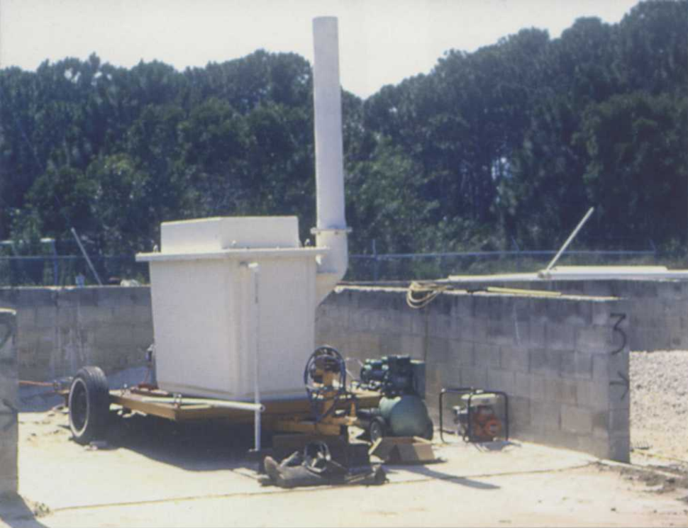
Contaminated groundwater requires special equipment like this stripping tower to remove residual material.
