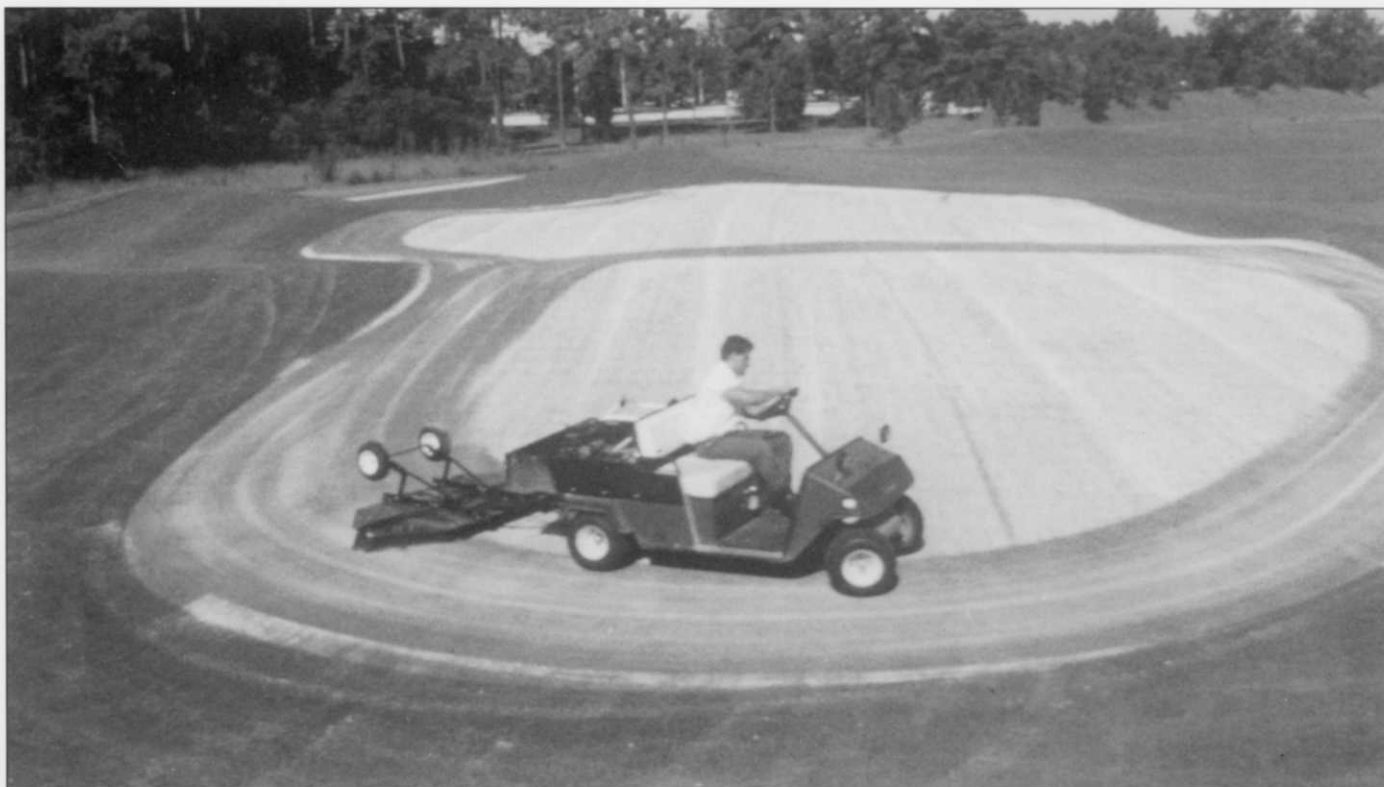
Dan Koronka uses a pull-behind drag brush to work the topdressing into the turf.
