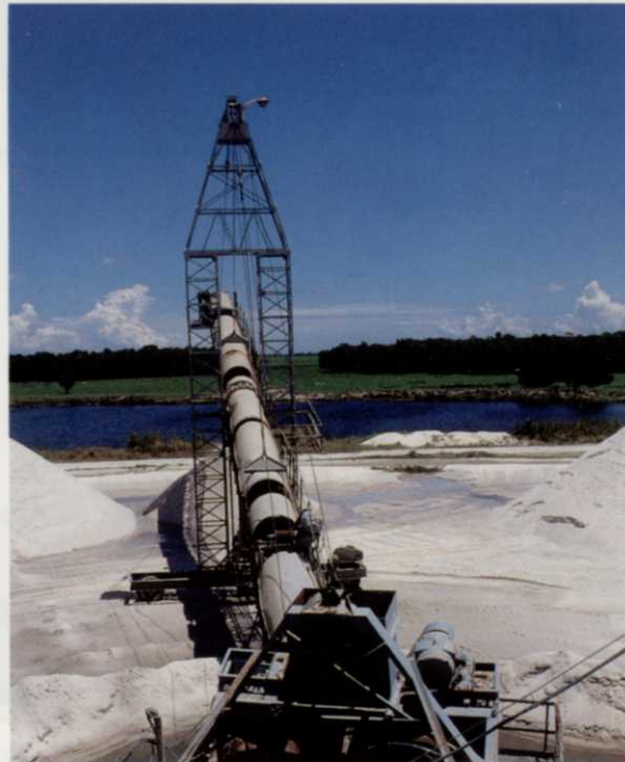
Conveyer can be rotated around the washer to stockpile sand once it has been screened and washed.
