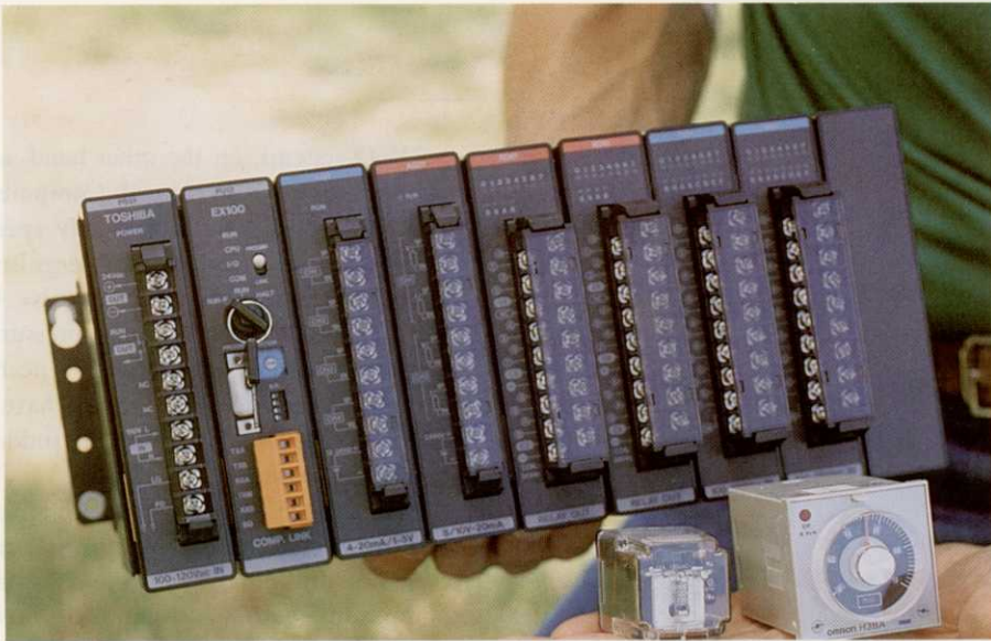
Most VFD pump systems use programmable logic controllers to store and manage information. The PLC above stores 165 pages of powerful computer code and can do the work of 99 conventional timers and 372 relays, such as those at bottom right of photo.
