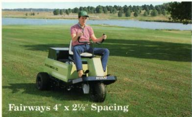
Now you can deliver "greens-quality" aeration to your entire course with a single piece of equipment. Variable core spacing makes the GA 30™ aerator as good on fairways as it is on greens. Simply move the spacing adjustment control from 1"-5" or anywhere in between, lock it in place, and you're ready to go without leaving your seat.
