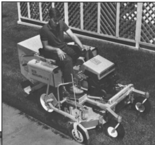
The 20 hp Hustler 251K with 51" Turbo Shredder™ mower deck, BAC-PAC™ and edger attachment.
