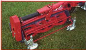
Fixed cutting unit, with anti-scalp rollers.
