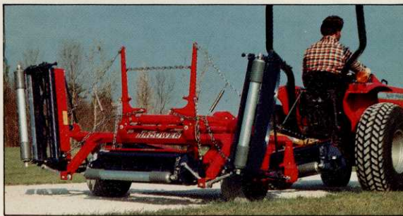
2. Hydraulic lift for easy transport or storage
