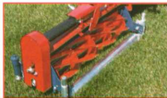
Floating cutting unit with front roller
