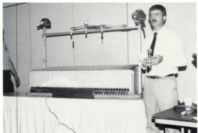
Dr. Curry demonstrates the effects of nozzles and spacing on precision coverage.
