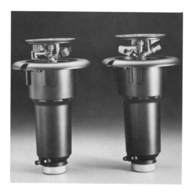
The 47DH and 51DH models have been engineered to stand up to the most demanding water quality conditions. The rotors feature a low pressure loss diaphragm valve, an energy efficient "straight-through" impact rotor drive, a self-flushing valve seat, and a long lasting, high strength plastic case.
