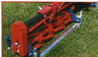
Floating cutting unit with front roller
