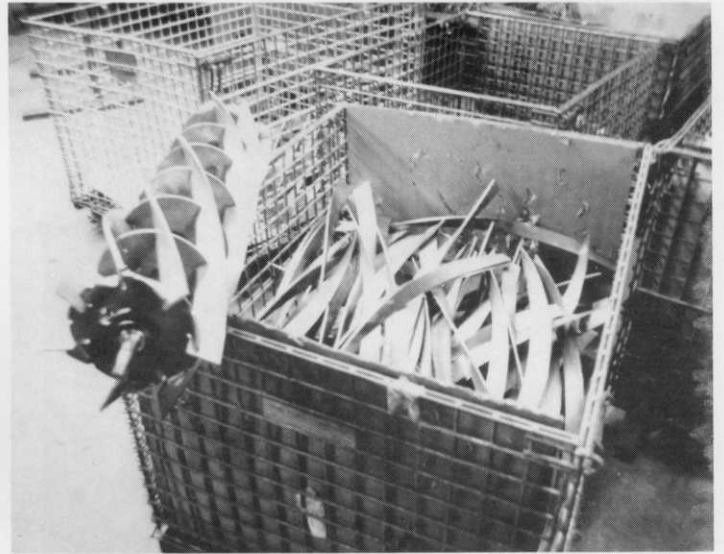
A bin of blades will ultimately come together to form a reel.
