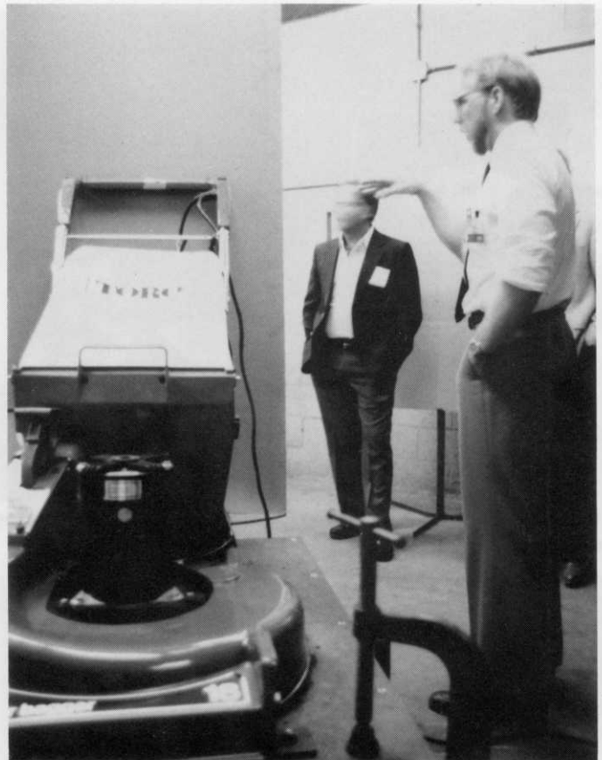
Metal leavings are injected into a whirling blade for shatter testing.
