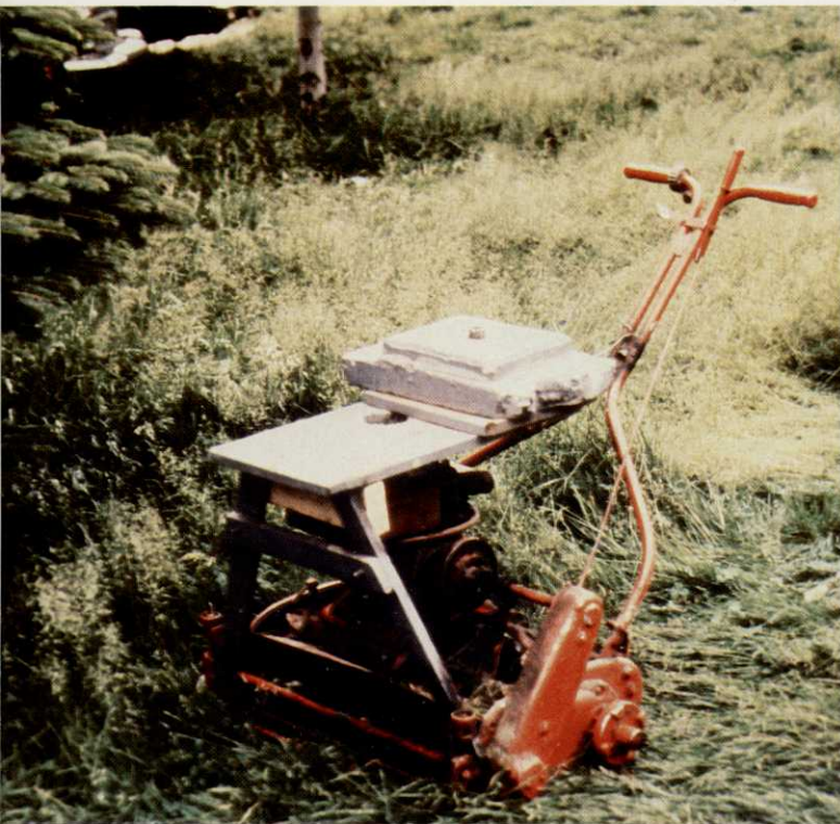
Some superintendents will add weights to their greens mowers for faster green speeds.
