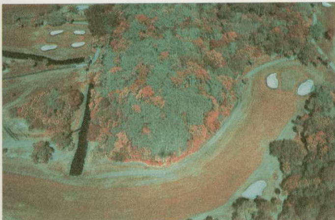
Dark streaks across the fairways at Hole-in-the-Wall in Naples, indicate underground lateral water flow and the direction of flow which was unknown at the time.
