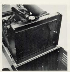
**EXTRA CAPACITY COOLING SYSTEM:** Groundsmaster 217-D has an industrial type radiator with tube and fin construction; 7 fins per inch to reduce radiator plugging. 6 quart capacity.
