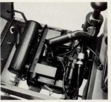
Groundsmaster 220 is powered by a 20 hp, 47.7 cu. in., twin cylinder, air cooled Onan engine for strong, quiet performance. Features include:
