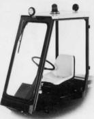
ROLL OVER PROTECTION SYSTEM. Certified roll over protection system (ROPS) for greater operator safety conforms to OSHA regulations, includes seat belt for greater safety.
