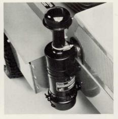
HEAVY DUTY DONALDSON AIR CLEANER is industrial type. Keeps your engine running longer by filtering out dirt and other contaminants before they can cause excessive wear. Allows dirt to be removed easily at the end of each day.
