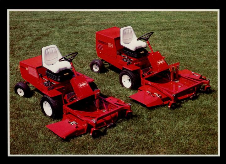
These durable riding rotaries, powered by air cooled gasoline or water cooled diesel engines, mow with exceptional maneuverability, trim close like walk mowers with a choice of 52" or 62" cutting units, and produce maximum results in a variety of applications.
