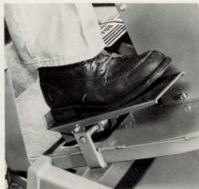
HYDROSTATIC DRIVE provides single pedal operation for forward/reverse speeds. Easy, smooth maneuverability with no clutch to wear out. Also, your operator gets superb speed control for all conditions. Infinitely variable speed up to 8.5 mph.
