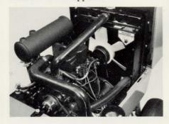
Groundsmaster 217-D has a 17 hp, 46.6 cu. in., water cooled Mitsubishi diesel engine. To protect the engine, standard features include high temperature shut down and oil pressure warning light/buzzer.
