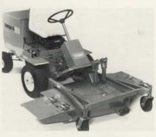
**CUTTING HEIGHT ADJUSTS EASILY** from 1 to 4 inches without tools. Simply pull four pins.
