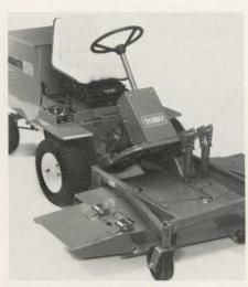
**P.T.O. DRIVE SHAFT** more efficient than most hydraulic drives, with mechanical engagement for decks or accessories. Avoids belt misalignments and makes changing from one accessory to another a breeze.
