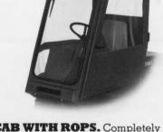
**CAB WITH ROPS.** Completely enclosed vinyl cab turns your Groundsmaster into an all-weather vehicle. Includes ROPS. Heater and light kit available.
