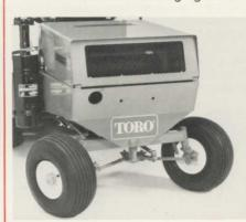
from 4 wide stance wheels plus low center of gravity. Front drive wheels and rear wheels are equipped with 4 ply rated tires. Both drive wheels have drum brakes controlled by individual pedals.
