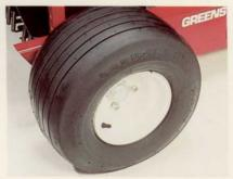
Larger floatation tires not only minimize compaction, they also make the machine easy to control.
