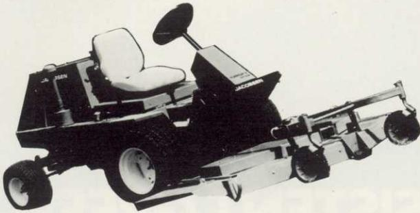
**THE JACOBSEN TURFCAT II DW224** is a new 4-wheel diesel, out-front riding rotary that features extensive use of hydraulics for simplified, reliable operation. Hydraulics drive the rotary, power the steering, lift the cutter deck and other implements, and operate the transmission. Jacobsen Turfcut II riding rotaries are also available in 3-wheel, rear steering models with gas or diesel engines.
