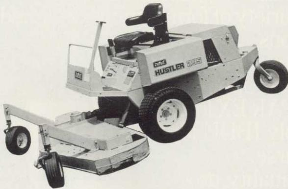
**THE EXCEL HUSTLER** is the most maneuverable of all out-front riding rotaries. It features a dual hydrostatic system that directs **INFINITELY VARIABLE** speed, direction, and braking through each drive wheel; all operated by one convenient hand control.
