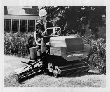
This extensively redesigned mid-size three-reel riding mower, introduced by DeBra Equipment Co., mows up to 33 ares of turf in one shift. The new Jacobsen Turf King II is available in either 76-in. or 84-in. cutting widths. Low-maintenance fetures include a 14 hp electric-start air-cooled engine, a large air filter with precleaner and a cooler operating hydrostatic transmission. ■
