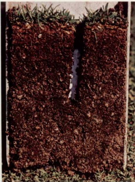
Greensaire II tines penetrate up to a full 3 inches.
