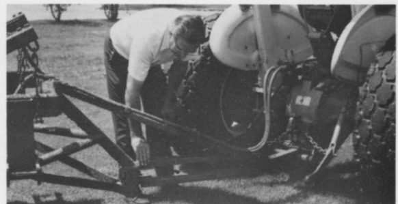
Healey's extension of hitch to keep fairway units from hitting tractor tire on turns.
