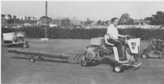
George Healey, Shop Superintendent demonstrates "reclaimed" Tri-Plex, hauling dragmat . . . also used to pull mat on green.
