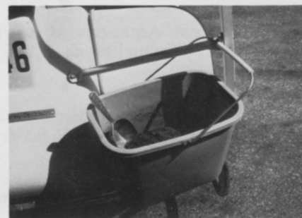
Buckets are attached to golf cars at convenient height, without getting in the way of golfers.
