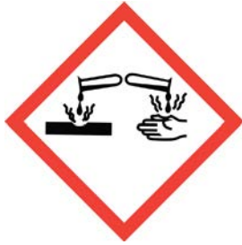
CORROSION Skin Corrosion/Burns Eye Damage Corrosive to Metals
