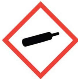
GAS CYLINDER Gases Under Pressure
