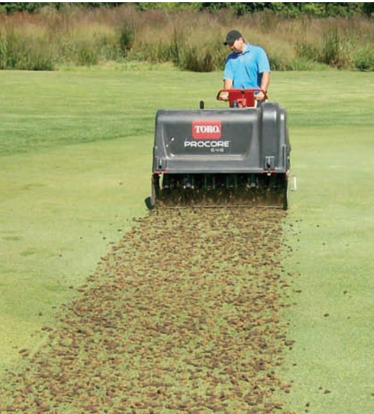
Cores are pulled and harvested from existing stands of bentgrass/Poa fairways and greens.
