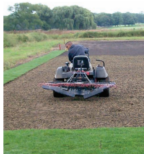
Using a sand rake tire tracks, the cores are then "dimpled" and prepared for a light seeding.
