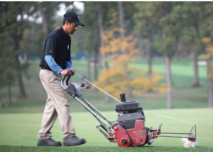
A retrofitted walking greensmower with brush combed the collars to create a difference in color of turf so the players could discern when they were on the putting surface.
