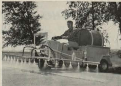
Spray rig can be equipped with specially-built boom which sprays 16-foot wide strip thoroughly and evenly. Variable-speed fast-acting governor insures correct speeds and even coverage on uneven terrain.
