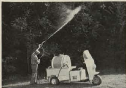
Specially-built spray rig is operated by Truckster engine through power take-off. Complete sprayer can be removed in minutes, freeing the bed for other loads, restoring the versatility of Truckster.
