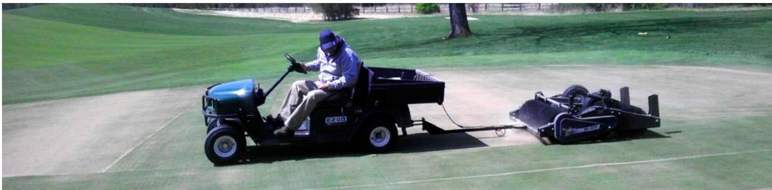
Incorporating sand with the T.B. 200 Brush. Photo Credit: Chuck Barber
