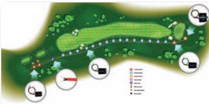
Possible hole design for a decoder system including block valves, single and multi station decoders, and communication/power line
