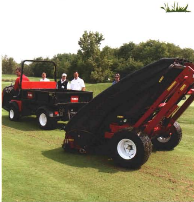
After lunch at the Field Day, an equipment demonstration took place. Pictured above is Toro's new Pro Sweep 5200 picking up aerification plugs on the Sunshine Course's 1st tee.
