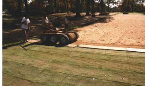
A customized installer for bigroll bentgrass sod.
