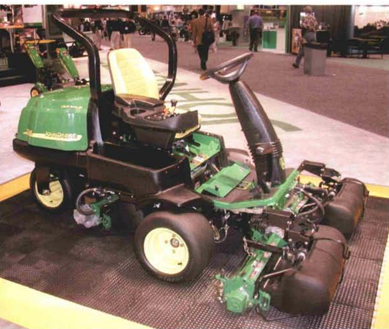
This is the 2500A minus hydraulic reel motors, hoses, lift valve etc. This unit eliminates 160 potential leak points.
