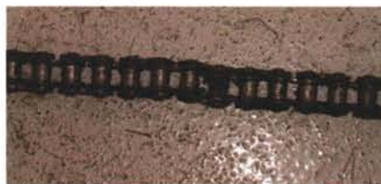
A chain with a damaged link.
