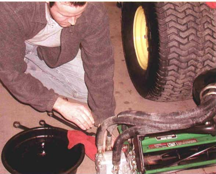
Inspecting hydraulic hoses for signs of wear is a key component of PM on a golf course.
